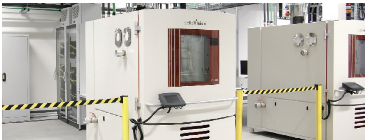
Battery test bench Source: Vollvision
